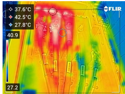
Scan the heat at the AC cable .
