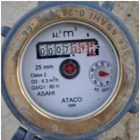
Water meter after cleaning
