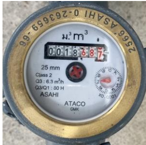
Water meter after cleaning
